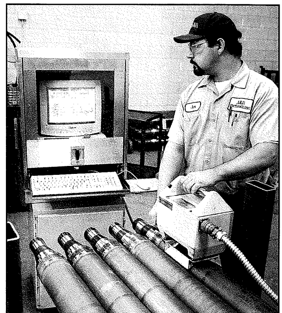
Pin stamp serial # on each beam and archive heat lot data for 100% traceability.
